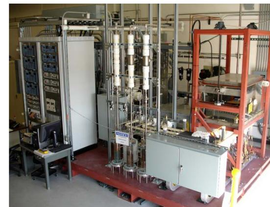
INL has demonstrated H<sub>2</sub> production rates up to 5.6 Nm<sup>3</sup>/hr in the ILS facility
